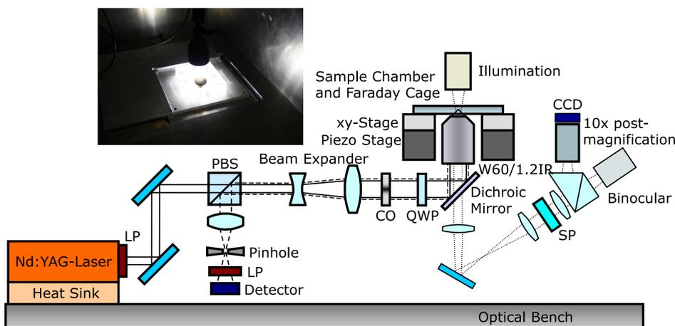
For illumination, we use a Schott KL2500 LED cold light source with a maximum output of 1000lm. Currently, due to contacting we cannot place the fiber directly onto the sample chamber. Therefore we focus the light with an additional lens.
